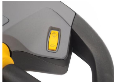
Two speed selector switch
